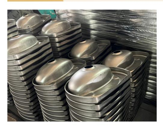
\*This image shows the working process of stainless steel wash basins. These wash basins are waiting to be lubricated and ground.
